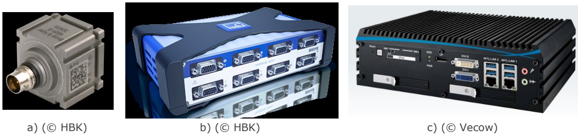
Figure 2: Vibration Sensor Measurement System
