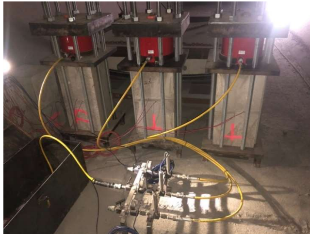
Figure 7: Koralmtunnel KAT3 - Test setup for in situ creep tests.
