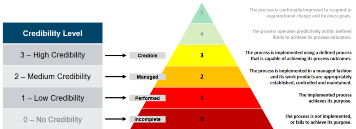
Figure 4: M&S SCPICE Process Capability Levels (ISO 2019; cf. [3])
