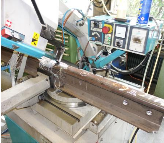
Figure 25: Test specimen and band saw during the cutting
