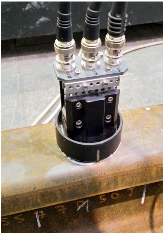
Figure 14: Ultrasonic test position on the upper side of the rail web
