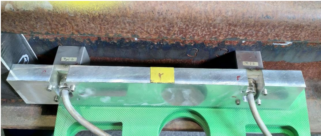
Figure 9: Transmitter-Receiver arrangement for Rayleigh wave measurement
