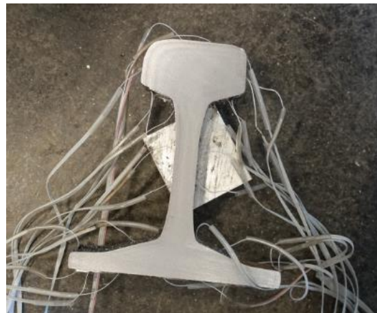
Figure 24: Cutted cross-section with strain gauges still attached
