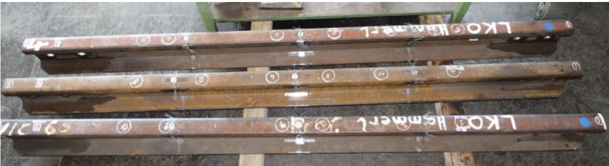
Figure 19: Prepared test specimen for the saw-cutting
