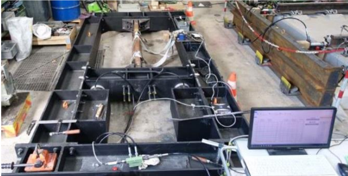
Figure 6: Mounted short test specimen loaded with compressive force
