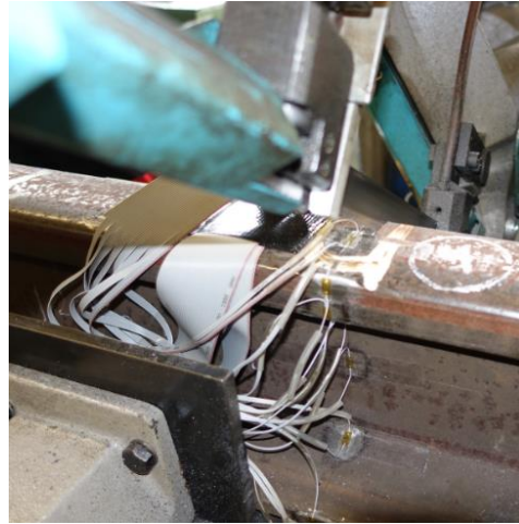
Figure 26: Detailed view of the cutting and strain gauges
