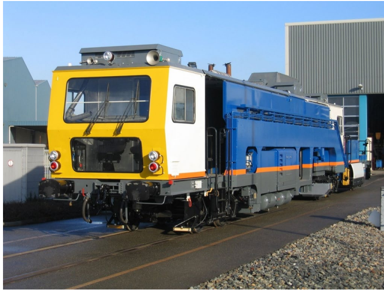
Figure 29 - Turnout measurement car with geometrical measurements [9]
